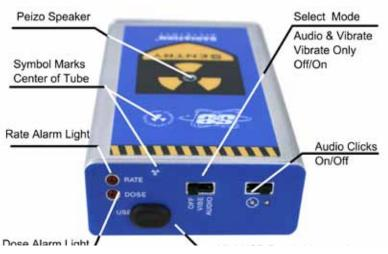
The rugged Alodized Aluminum Housing protects the unit in tough industrial environments
