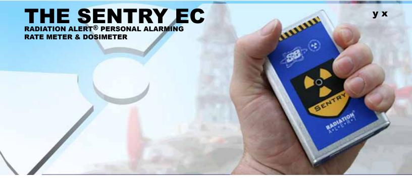
The Radiation Alert<sup>®</sup> Sentry EC is a Personal Alarming Dosimeter / Ratemeter designed to ensure the safety of personnel that work in occupations with potential x-ray or gamma exposure.
